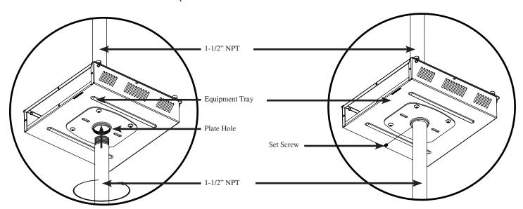
**Step 1.** Place the threaded end of the 1-1/2" NPT into the plate hole.
